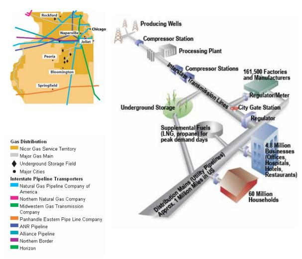
Fig. 18. Gas distribution and pipeline system. (Nicor Gas, 2009)
