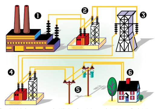
When electricity leaves a power plant (1), its voltage is increased at a "step-up" substation (2). Next, the energy travels along a transmission line to the area where the power is needed (3). Once there, the voltage is decreased, or "stepped-down," at another substation (4), and a distribution power line (5) carries the electricity until it reaches a home or business (6).
